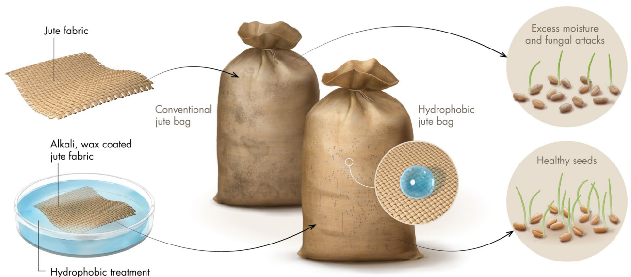
Figure 7. Schematic showing the surface treatments of jute bags with alkali and wax coating, the seed storage experiment, and the germination experiment for stored wheat grains. Control jute bags, CJBs; hydrophobic (wax-coated) jute bags, WCJBs. While CJBs accumulate water and get wet, WCJBs prevent water accumulation and cause water droplets to roll off their surface. Post-storage seeds from WCJBs are more likely to have higher germination than seeds from CJBs (image credits: Xavier Pita, KAUST).
