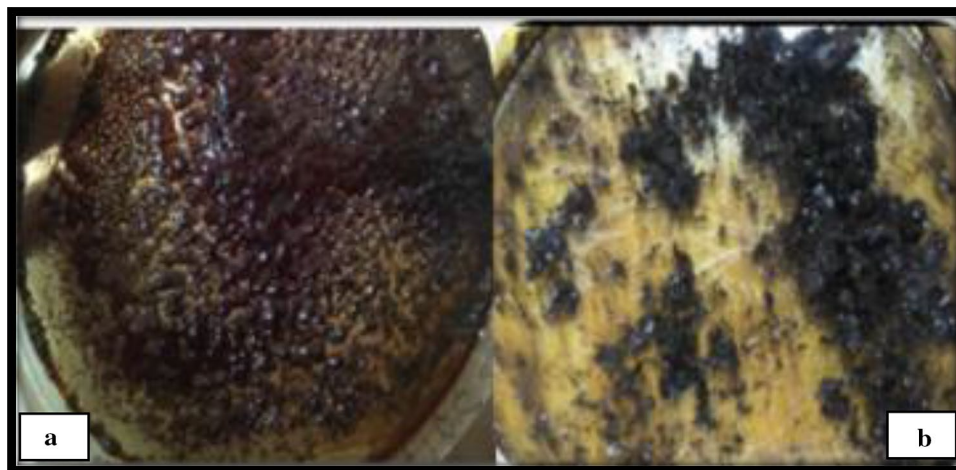
Figures 1. (a) Wet Cadmium oxide-extract moiety in the oven, (b) Dried CdO/CdCO 3 NPs.
