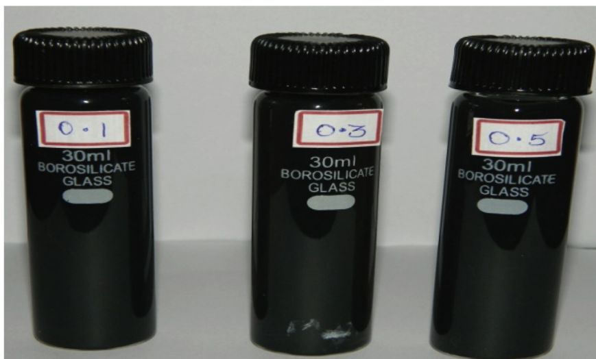
Fig. 3. Photograph of MWCNT/water nanofluids 45 days after preparation.
