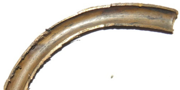
Fig. 12. Assessment of deposit of MWCNTs on coiled tube after conducting tests.
