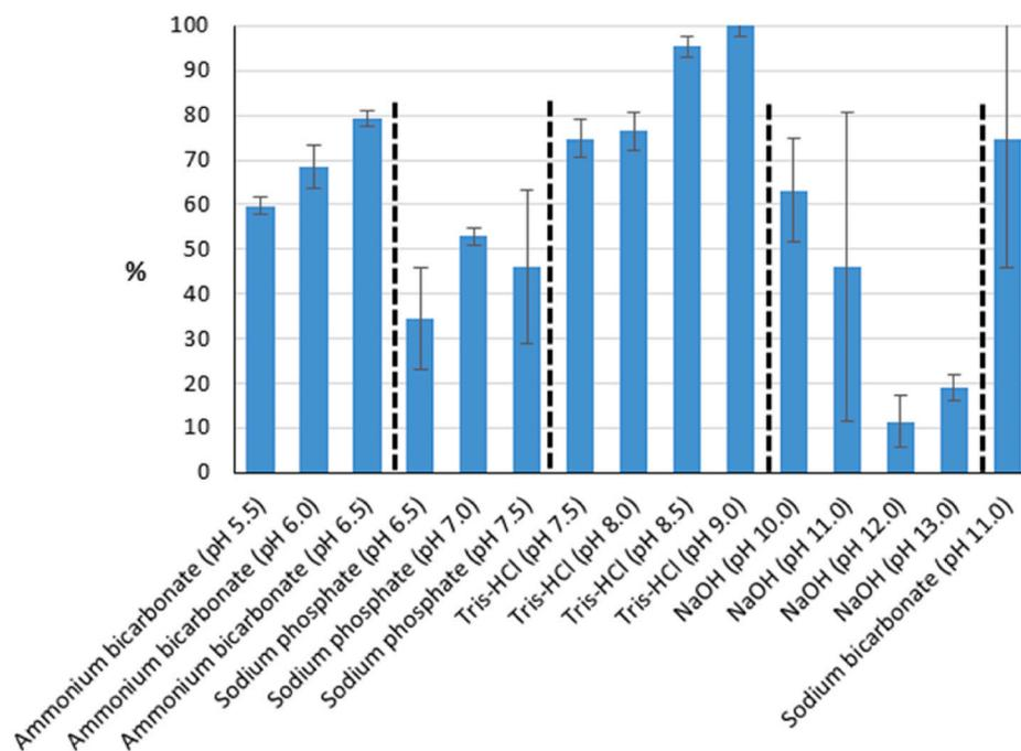
Fig. 1. Relative recovery of proteins obtained at different pHs and buffers using UAE. Other experimental conditions were: 30% of ultrasounds amplitude, 5 min extraction time, and room temperature.
