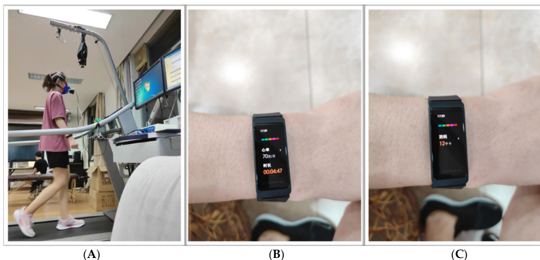
Figure 1. A subject walked on a treadmill with one bracelet on each wrist (A), monitoring heart rate (B) and energy expenditure (C), respectively.
