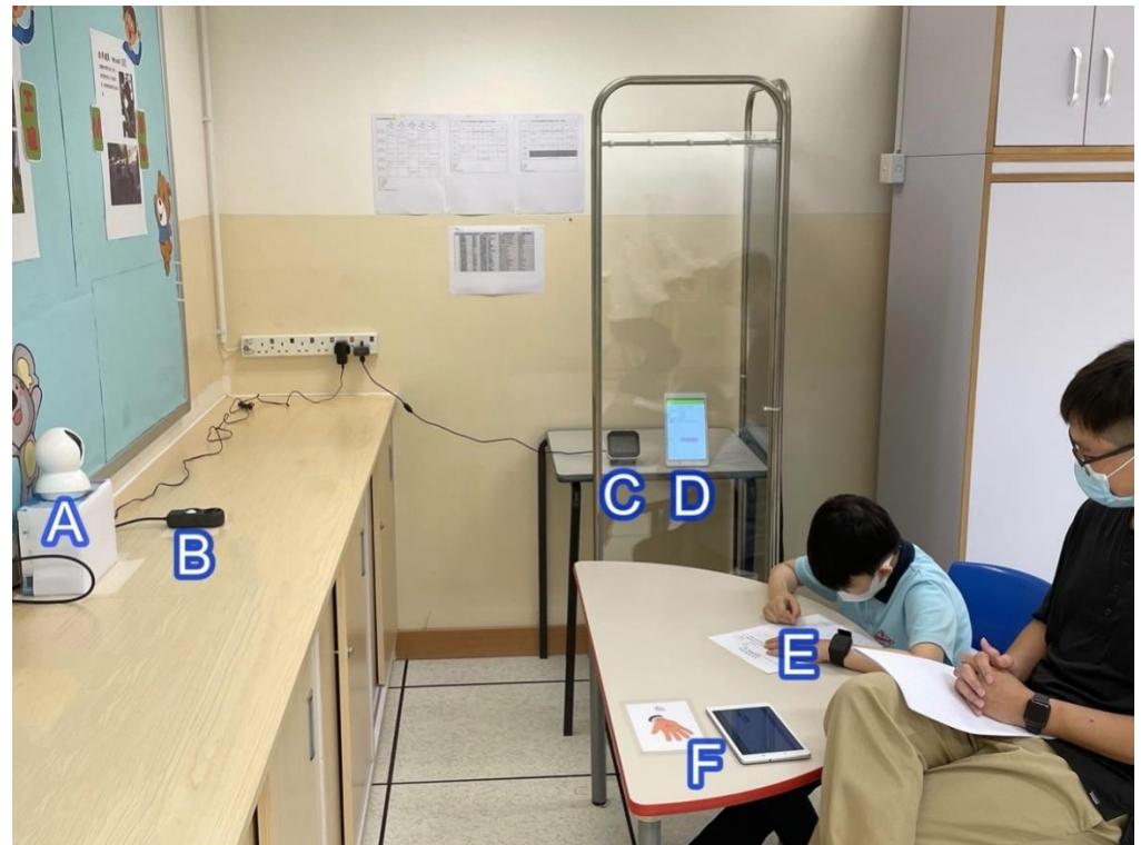
Figure 2. The SEN classroom serving as the context of our student-centered learning environment where IoT-enhanced ABA was delivered. (A) Camera; (B) Light Sensor; (C) CO 2 /Humidity/Temperature Sensor; (D) Emotion Recognizer; (E) E4 wristband; (F) mobile client of the 3i-Learning System.
