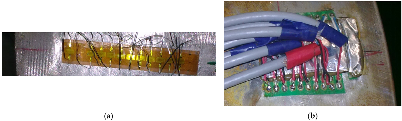
Figure 6. Photographs of strain gauges chain glued on tested pressure vessel: (a) strain gauge before connecting the wires; (b) finished connection.
