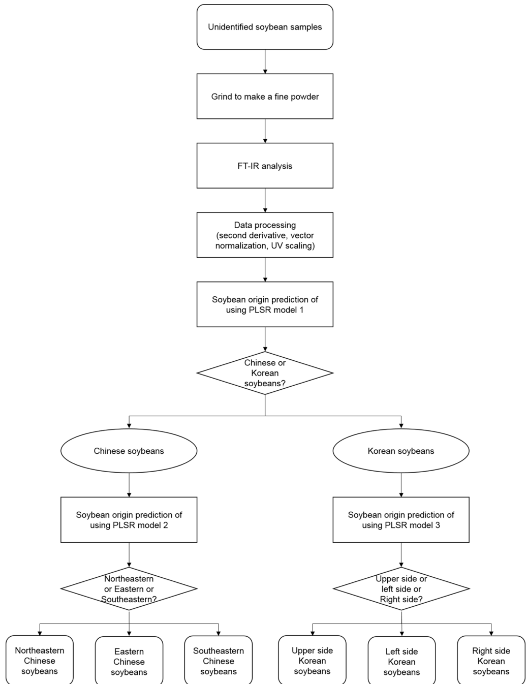
Fig 6. Flow chart for discrimination of unidentified soybean origin using FT-IR.
