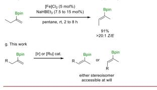
Reinsertion of the hydride would result in the formation of the *E*-alkenylboronate ester. Notably, overisomerization leading to allylboron species should be avoided due to the substitution pattern of the alkenylboronate substrates employed and the reluctance of the 1,3-hydride shift-based catalyst to generate allyliridium hydride intermediates featuring branching at the termini.
