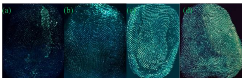
Figure 3. Fingermarks developed by G-CDs on various substrates. (a) sealed bag; (b) coverslip; (c) transparent tape; (d) tin foil paper.
