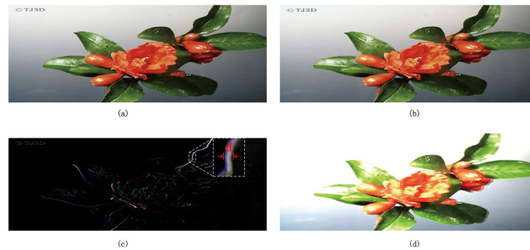
Fig 3. Summation and difference of stereo pair (a) Left view, (b) Right view, (c) binocular difference map and (d) binocular summation map.
