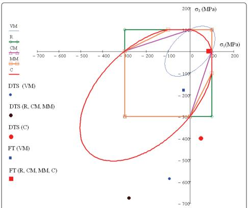
**Figure 4 Failure lines for different criteria and location of critical points for DTT and FT.** Failure lines for the different failure criteria in a planar stress condition ( $\sigma_2 = 0$ ) in a plot of maximum principal stress  $\sigma_1$  against minimum principal stress  $\sigma_3$ , for a hypothetical brittle material with TS = 100 MPa and CS = 300 MPa, together with the location of the critical points for DTT and FT with the different failure criteria.
