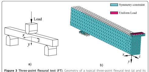
corresponding FE mesh with two planes of symmetry (b).
