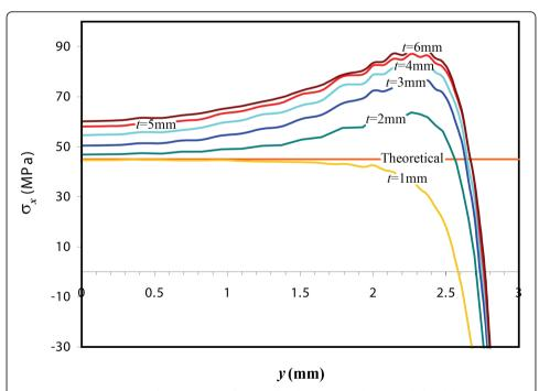
**Figure 6** Normal stress in the x-direction for DTT for the exterior diameter defined by z = t/2, x = 0. Normal stress in the x-direction,  $\sigma_{xx}$  along the line defined by z = t/2, x = 0, y = [0, D/2] for the six DTT models with thicknesses from 1 mm to 6 mm, and the theoretical result obtained with the plane stress hypothesis.
