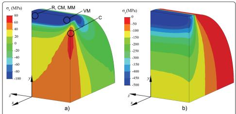
**Figure 5 Normal stress in the x-direction and y-direction in DTT.** Normal stress distribution in the x-direction (a) and y-direction (b) obtained in DTT for a disc thickness t=3 mm, and location of predicted failure initiation areas for different failure criteria (a).
