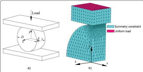
**Figure 2 Diametral tensile test (DTT).** Geometry and parameters of a typical diametral tensile test on a cylindrical specimen of a brittle material (a), and its corresponding FE model with three planes of symmetry (b).
