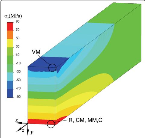
**Figure 7 Normal stress in the z-direction for FT.** Normal stress in the z-direction for the three-point flexural test simulation, and location of predicted failure initiation areas for different failure criteria.
