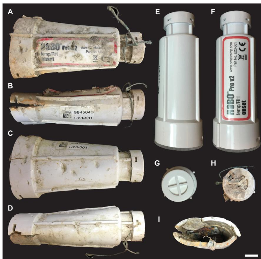
**Figure 2** Damaged and pristine Onset HOBO Pro v2 Temp/RH (U23-001) data loggers. (A–D) Damaged data logger from four angles, representing the full circumference of the device. Bite marks and evidence of compression and cracking are present in all four views. (E–G) Pristine data logger in side and top views. (H–I) Damaged data logger in top and bottom views, showing the degree of compression and cracking in the damaged device. Scale bar = one cm.
