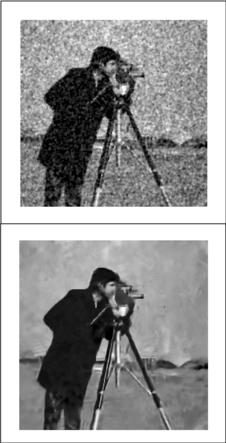
Figure 17 Results of our method (up) and BM3D technique (down) with SNR = 75 for Cameraman.
