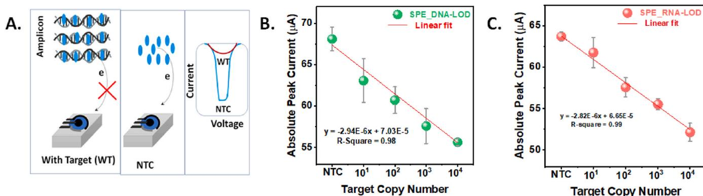
Fig. 3. Electrochemical LAMP studies conducted on pure  $10^1$ – $10^4$  copies of SARS-CoV-2 *RdRp* plasmid DNA (Panel B) or RNA/reaction (Panel C) (without magnetocapture). Panel A describes the mechanism of amplicon-mediated methylene blue sequestration and subsequent reduction of current. NTC assays were conducted without any template nucleic acid addition. (For interpretation of the references to color in this figure legend, the reader is referred to the Web version of this article.)
