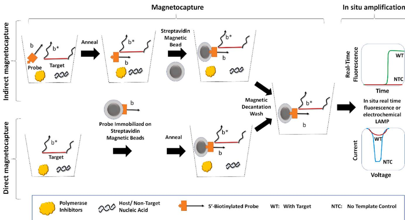
**Scheme 1.** Indirect and direct sequence-specific magnetocapture of target nucleic acid (present with host nucleic acid and polymerase inhibitors from serum) leads to probe-target nucleic complex immobilized on the magnetic bead. Following magnetic decantation wash, the target bound magnetic beads was used for in situ LAMP (or reverse transcriptase LAMP) amplification with fluorescence or electrochemical readout.
