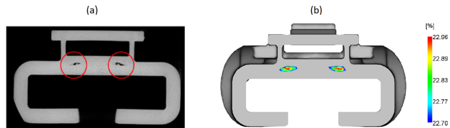
Figure 12. Location of the voids: (a) 3D X-ray slice of FH part, (b) Prediction of volumetric shrinkage at the void locations.
