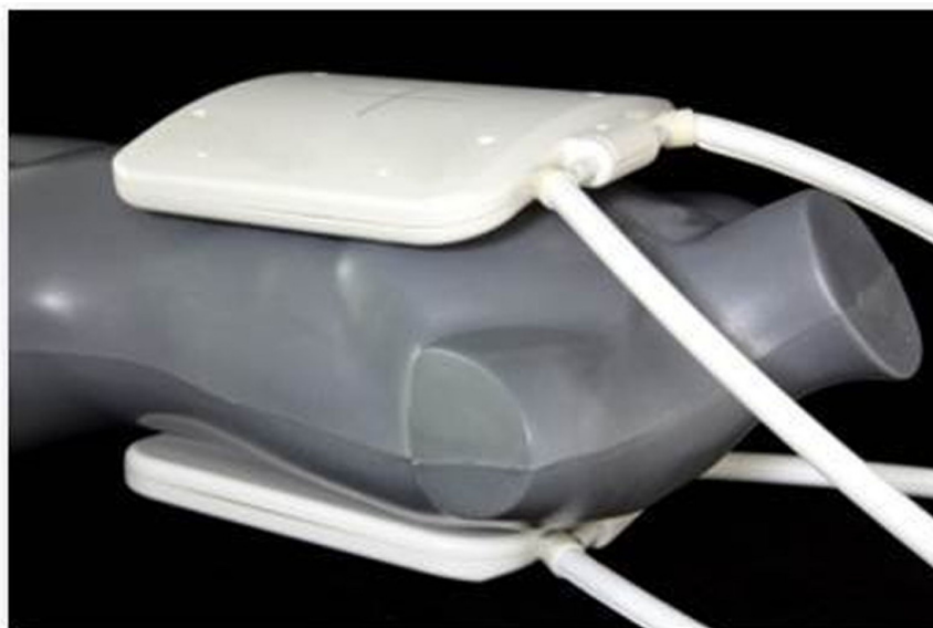
Figure 1 The coil housed in two modestly curved lightweight formers to conform to an average chest and back, shown on a mannequin.
