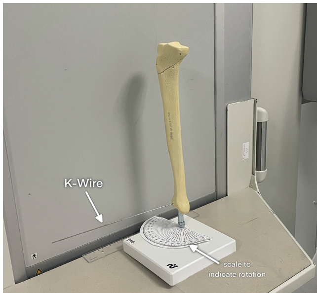
Figure 2. Experimental setup: the saw bone model was positioned in front of the x-ray detector plate. A K-wire was fixed at the level of the distal tibia to indicate the change in rotation on a scale. The fixation of the saw bone to the base-plate allowed for adaptation of the rotational alignment.
