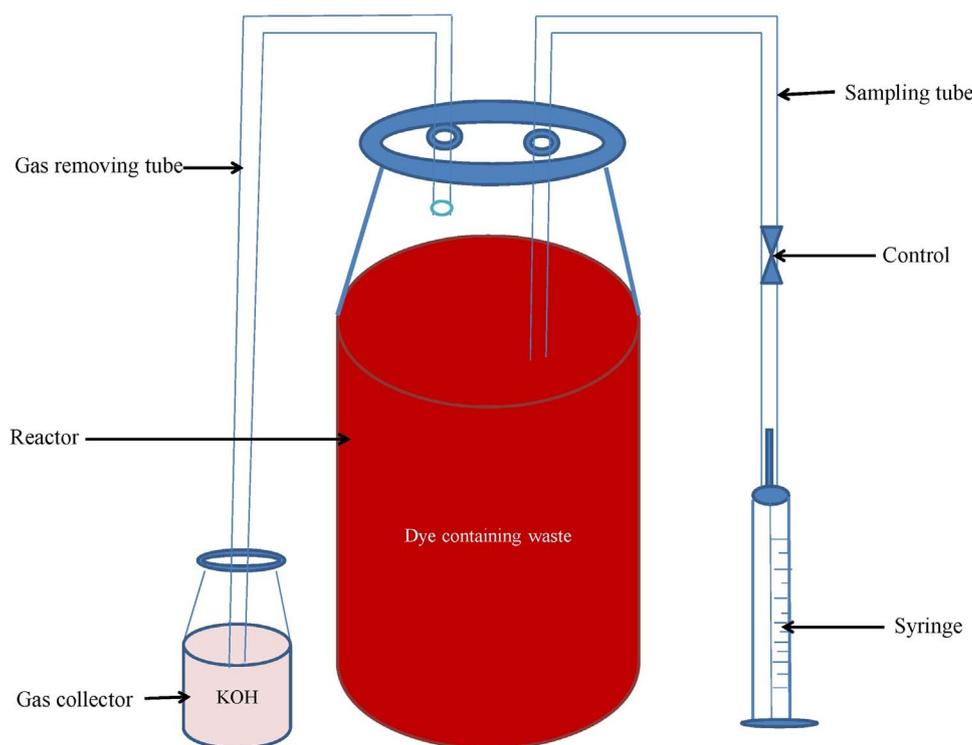
Fig. 1. Schematic of the decolorization reactor setup.
