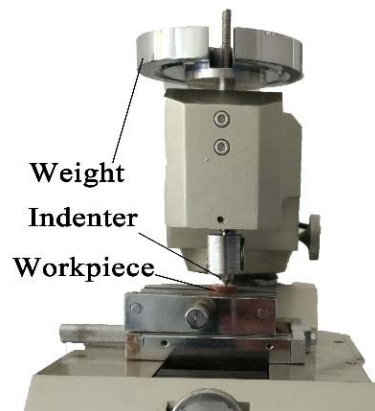
Figure 7. Experimental set-up of the friction coefficient.
