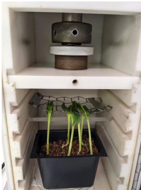
Figure 4. Maize variety Golden Bantam seedlings in the chamber of the PDS-1000/He biolistic particle delivery system
