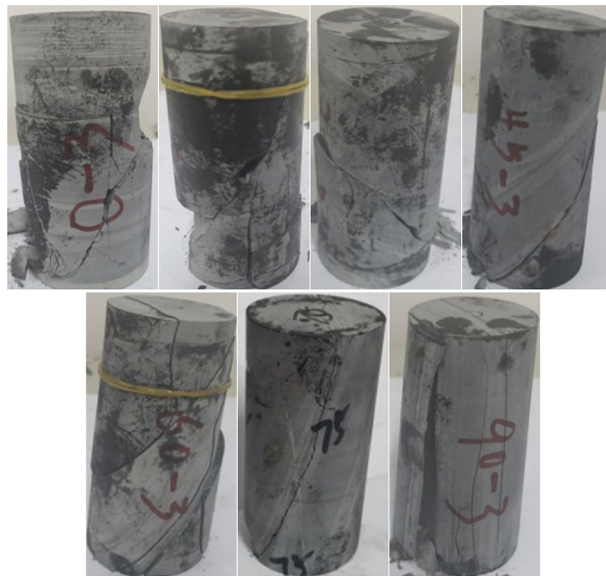
Figure 7. Macroscopic destruction picture of Phyllite.
