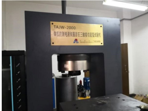
Figure 2. TAJW-2000 triaxial shear rheometer.
