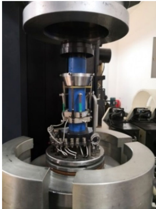
Figure 3. Sample installation diagram.
