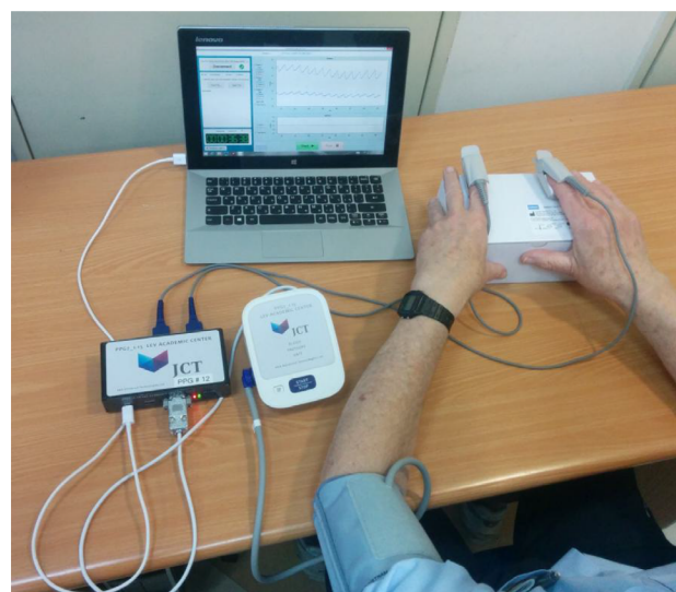
Figure 1 The PPG-based SBP measurement apparatus includes a pressure cuff wrapped around the arm and two photoplethysmographic probes on the fingers of the two hands.
