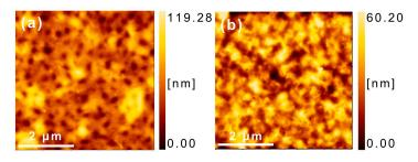
**Figure 6.** Atomic force microscopy (AFM) height images (5  $\mu$ m × 5  $\mu$ m) of (**a**) P3HT/P(NDI2OD-T2) and (**b**) P3HT-*b*-PSt/P(NDI2OD-T2)-*b*-PSt.
