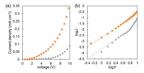
**Figure 4.** Current density-voltage (**a**) and double logarithmic plots (**b**) for electron only devices based on P(NDI2OD-T2) (gray) and P(NDI2OD-T2)-*b*-PSt (orange). The presented data set affords the electron mobilities close to the average values.
