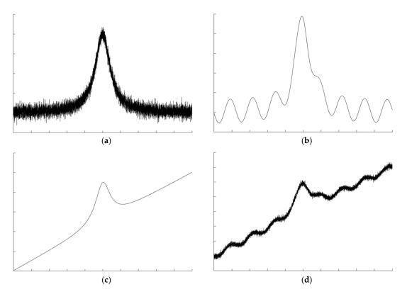
**Figure 1.** Signal simulation. (**a**) White noise; (**b**) interference fringe; (**c**) background; (**d**) multiple interference signal.
