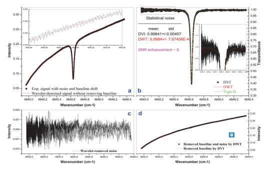
**Figure 14.** (a) Experimental spectrum of  $CO_2$  (pressure = 140 mbar; path length = 4800 cm; mixing ratio = 1.0%; temperature = 292.95 K) and wavelet–denoised signal; (b) Baseline drift removed transmittance signals using DVI and DWT, as well as the Voigt fit; (c) DWT removed noise; (d) DWT removed baseline with noise and DVI removed baseline. Parts of the "baselines" are expanded for clarity and statistical noises are also provided in the inset. This figure was obtained from [52].
