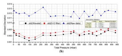
**Figure 6.** (a) Raw signal and processed signal by wavelet and S–G filter under different noise level. (b) Standard deviations of three sets of data under different pressure. This figure was obtained from [41].
