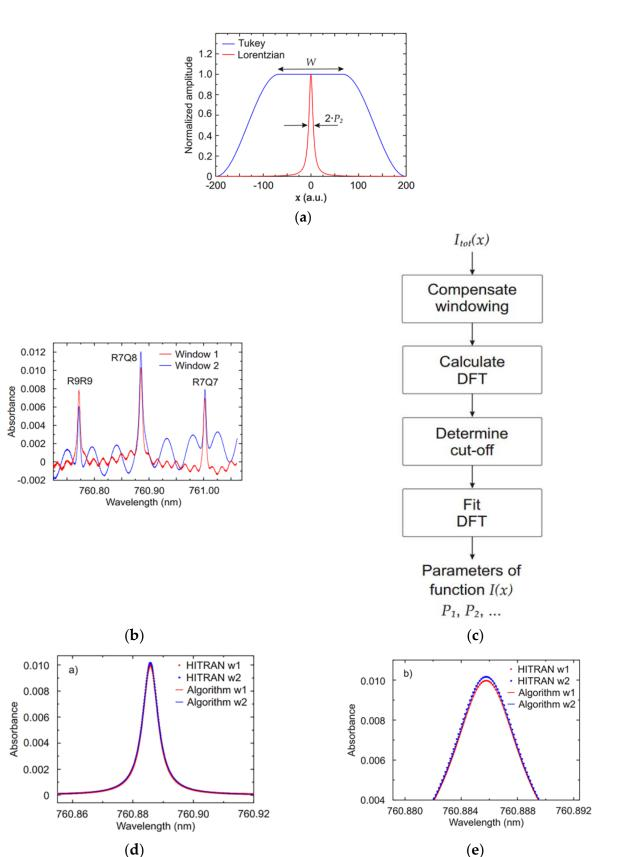
**Figure 10.** (a) Tukey window; (b) deliberately made interference fringe, (c) algorithm flowchart, (d) experimental result, (e) detail of the processed signal. This figure was adapted from [36].
