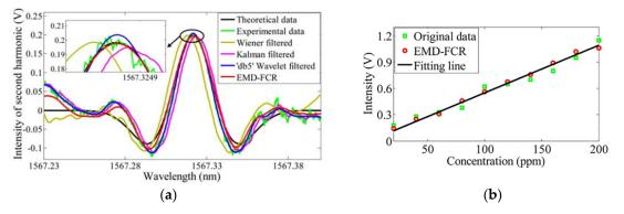
**Figure 8.** (a) Performance of different methods. (b) Relationship between the second harmonic intensity and gas concentration. This figure was obtained from [42].
