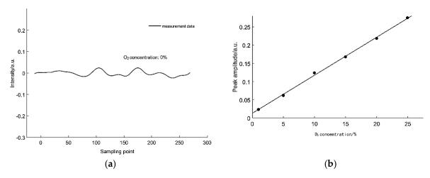
**Figure 9.** (a) Zero concentration fringe. (b) Relationship between the peak amplitude and gas concentration. This figure was adapted from [47].
