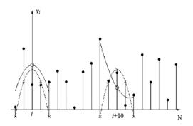
**Figure 4.** Illustration of least-squares smoothing by locally fitting a low-order polynomial (solid line) to five input samples: dot denotes the raw input samples, circle denotes the least-squares smoothed samples, and x denotes the effective impulse response samples. The dotted line denotes the polynomial approximation to centered unit impulse. This figure was taken from [41].
