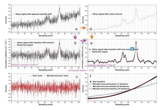
**Figure 13.** Nonlinear baseline correction and denoising using DWT. (**a**) Noisy signal with apparent baseline drift; (**b**) baseline drift removed signal from (**a**) and noise-free signal; (**c**) raw noise and wavelet-removed noise; (**d**) denoised signal from (**a**); (**e**) baseline drift removed signal from (**d**) and noise-free signal; (**f**) raw baseline and wavelet-removed baseline. This figure was obtained from [52].
