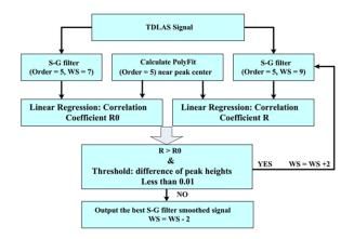
Figure 5. Flow chart of adaptive Savitzky–Golay algorithm. This figure was adopted from [41].
