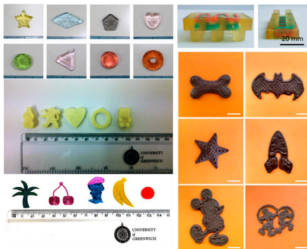
Figure 3. 3D-printed solid dosage forms for pediatric patients; gummy dosage forms ( upper left ) [41]; dosage forms shaped like candy (Starmix ® ) ( middle left ) [42]; taste-masked chewable dosage forms in various shapes ( lower left ) [43]; soft chewable Lego ™ -shaped dosage form ( upper right ) [44]; chocolate-based dosage forms in various shapes ( lower right ) [40].
