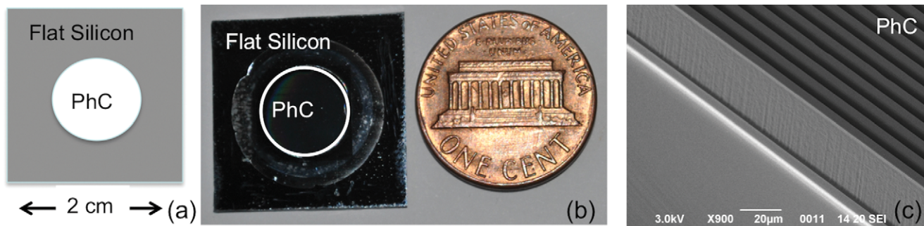
Figure 1. Images of silicon devices. a: Schematic drawing of the different regions on a silicon chip. b: Photo of the device together with a reference size. c: Scanning Electron Microscopy image of the three-dimensional silicon microstructure. doi:10.1371/journal.pone.0048556.g001
