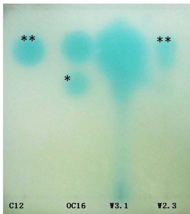
Figure 4. Thin layer chromatography analysis of AHLs. AHL standards from Sigma (C12-HSL (**)) and 3-oxo-C16-HSL (*) and 10 \mu l of W3.1 and W2.3 extract were spotted on normal phase TLC plate. The TLC plate was chromatographed with dichloromethane and methanol as mobile phases. The locations of AHLs were revealed by overlay of Agrobacterium tumefaciens NTL4 pZLR4 as evident by blue pigmentation. Based on the R_f values, W2.3 produced C12-HSL. doi:10.1371/journal.pone.0044034.g004
