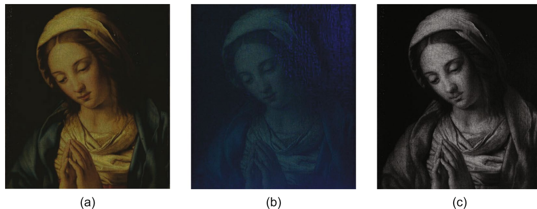
Figure 1. Images of Madonna in Preghiera . (a) Visible photograph of the Madonna in Preghiera ; (b) Image of Madonna in Preghiera obtained by UV Fluorescence; (c) Image of Madonna in Preghiera obtained by IR Reflectography.
