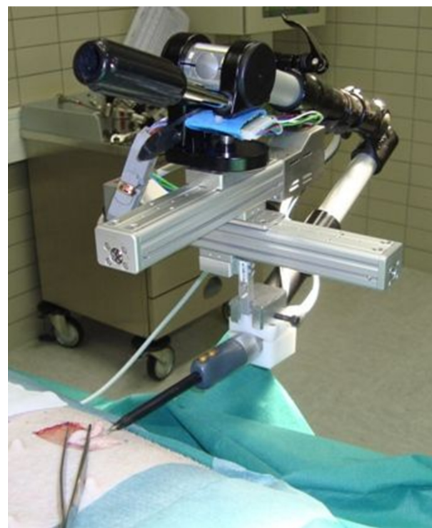
Figure 1 Automatic device for soft tissue dissection. Self-constructed apparatus fixed at the operating table and loaded with ultrasonic scalpel. The instrument can be moved engine-driven into two directions (aluminium tracks).
