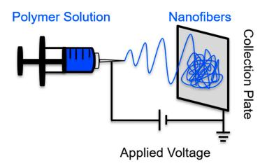
**Figure 1.** The cartoon displays the basic electrospinning process, including a high voltage supply and a syringe/needle that is held at a fixed distance from a collection plate. To control the polymer solution flow rate, an advancement pump is typically used. Adapted, with permission, from Meng et al. [35].
