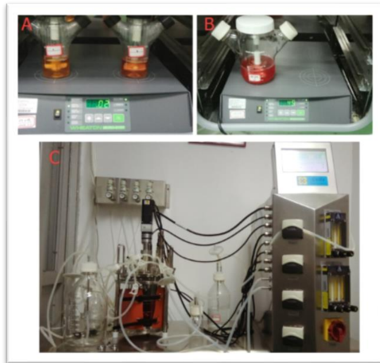
Figure 2. Different suspension culture systems. (A) The 125 mL stirring flask; (B) the 500 mL stirring flask; (C) the 3 L bioreactor.
