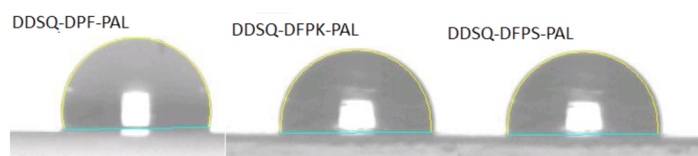
Figure 9. Water contact angles of DDSQ-DFPXs-PAL films after curing.
