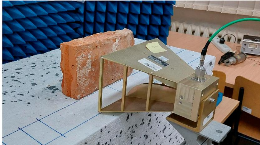
**Figure 3.** Close up of the laboratory setup during microwave measurements: double ridge antenna, a brick, styrofoam stand and microwave absorbers.
