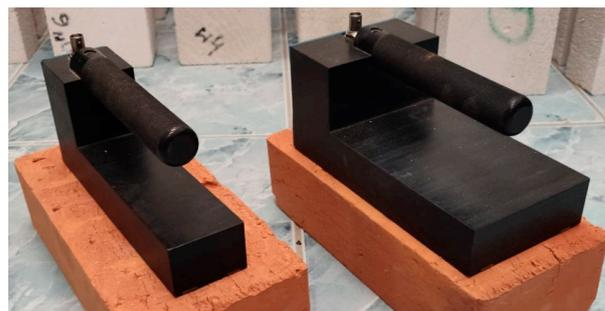
**Figure 2.** Photograph of non-invasive TDR sensors—Sensor A (left), Sensor B (right).
