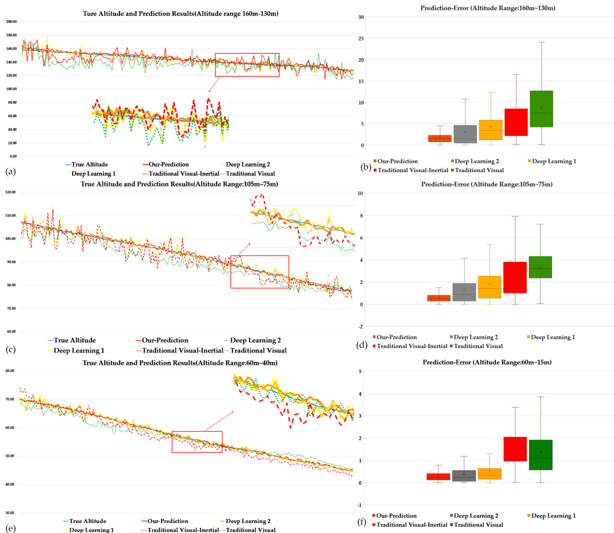
Figure 8. The comparison of all methods' prediction results and the prediction–error. (a) shows the prediction results of all the methods in altitude range from 160 m to 130 m. (b) shows the prediction error of all the methods in altitude range from 160 m to 130 m. (c) shows the prediction results of all the methods in altitude range from 105 m to 75 m. (d) shows the prediction error of all the methods in altitude range from 105 m to 75 m. (e) shows the prediction results of all the methods in altitude range from 60 m to 40 m. (f) shows the prediction error of all the methods in altitude range from 60 m to 40 m.
