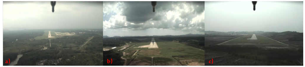
Figure 6. The images captured at different flight altitudes during the UAV landing phase. (a) The image is captured in the altitude range of 160~110 m. (b) The image is captured in the altitude range of 105~75 m. (c) The image is captured in the altitude range of 70~40 m.
