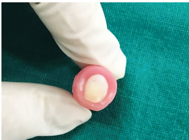
Fig. 2: Mounting of the test sample in the acrylic block
