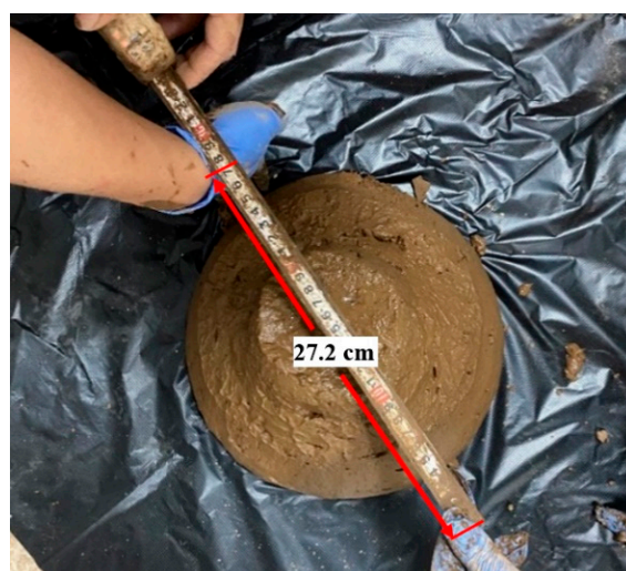
Figure 3. Measurement of slurry expansion with a mass fraction of 64%.
