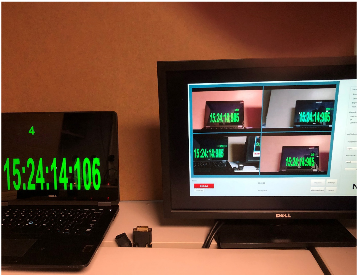
Fig. 10. A close-up image from the experimental setup shown in Fig. 1. The image highlights the synchronicity of all four RPi cameras. It is clear from the DVR GUI that all four RPi are displaying the same frame counter number (i.e., the '29' shown above the hr:min:sec:msec reading) of the clock being video-recorded by the RPi's. The image also shows the latency between the preview and the clock being recorded. Namely, the clock is on frame 4 whereas the preview is on frame 29 of the previous second, amounting to a 5-frame delay or approximately 167 ms preview latency.
