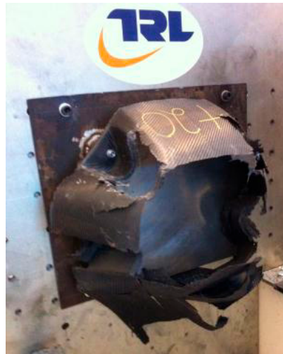
Figure 9. Carbon fiber nose cone after impact [18].
