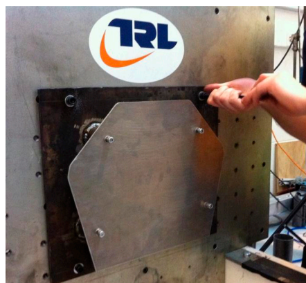
Figure 8. Nose cone mounting plate—showing 50 mm offset [18].
