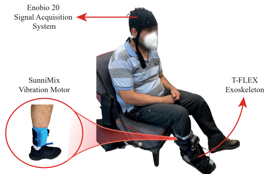
Figure 4. Experimental system setup for BCI-based control using T-FLEX with visual and haptic stimuli.
