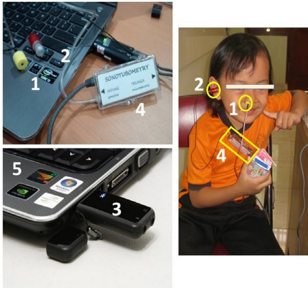
Figure 1. Sonotubometry device: 1. Hearing Aid speaker (ear tone 3A); 2. Type CM 120 condenser microphone; 3. SB1140 creative sound card; 4. SN 002020; 5. Laptop.
