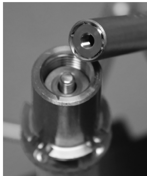
Figure 9 After the spindle with the appropriately sized centering sleeve is placed over the anchor plug traction bar, compression must be applied. This is achieved by tightening the nut over the washers inside the spindle. (The compression cap is not shown.)
