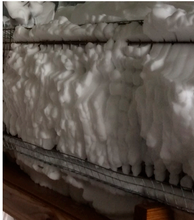
Figure 2. Cages filled with compressed air foam.
