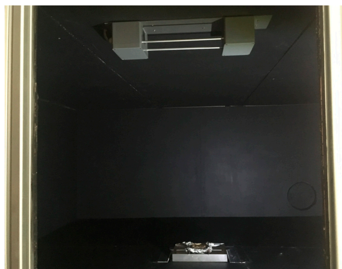
Figure 10. The interior of a reduced-scale (1:4) chamber with visible reduced-scale optical densitometer mounted underneath the ceiling.
