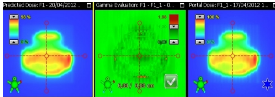
FIG. 2. Predicted fluence (left) for a modulated field reconstructed according to the DynaLog files. The gamma analysis (middle) shows that the DynaLog-based method is accurate enough to reproduce the delivered fluence (right).
