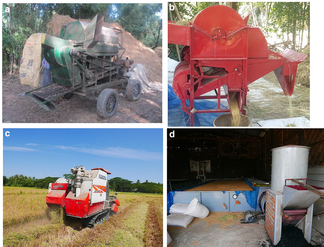
Figure 2. (a) Farmer thresher. (b) Imported thresher, TC-800. (c) Combine harvester Kubota-DC-70G. (d) Flatbed dryer 4 ton batch -1 .
