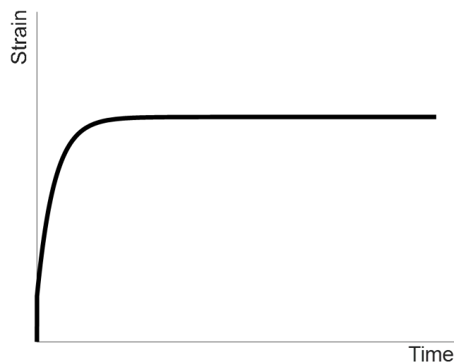
Figure 1. Illustration of creep behavior (increasing strain over time).
