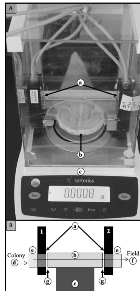
Fig. 2 Image (A) and schematic (B) of analytical balance showing pathway of bees from the colony to the field. Bees leave colony (d) via exit tube (e), pass through one RFID reader (a), navigate a maze (b) resting on the analytical balance, pass through a second RFID reader (a), enter a second exit tube (e), then depart into the outside environment (f). The maze allowed the balance to stabilize while the bee was on it. Small gaps (g) were necessary to ensure free movement of the scale surface. A motion-activated camera took short video clips of each bee on the maze, and the balance fed time-stamped weight data continuously to a computer
