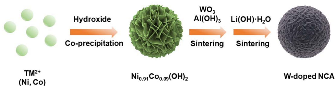
Figure 1. Schematic illustration of the preparation of W-doped NCA cathodes.
