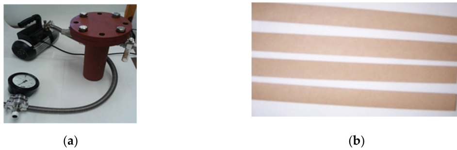
Figure 6. (a) Steel container and vacuum pump and (b) strips of Kraft paper.
